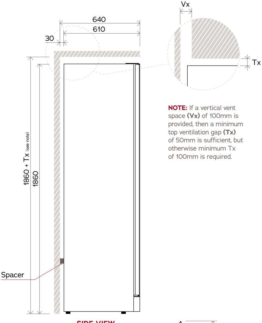
**NOTE:** If a vertical vent space (**Vx**) of 100mm is provided, then a minimum top ventilation gap (**Tx**) of 50mm is sufficient, but otherwise minimum Tx of 100mm is required.
